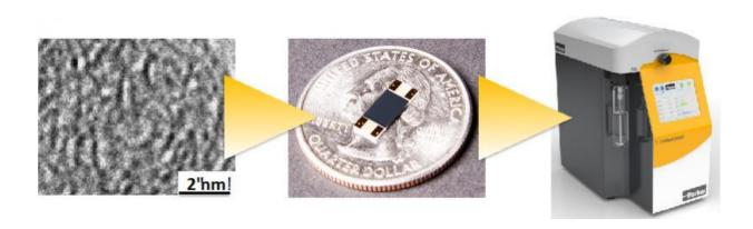
Transmission electron microscopy image of nanoporous carbon, left, "the most controllable carbon in the world, in the terms of its mass density and its total surface area," according to Sandia National Laboratories researcher Mike Siegal. A nanoporous carbon coated surface acoustic wave sensor on a quarter, middle. This sensor is the key component of Parker Hannifin's Trihalomethane Water Analyzer, right. Credit: Sandia National Laboratories
