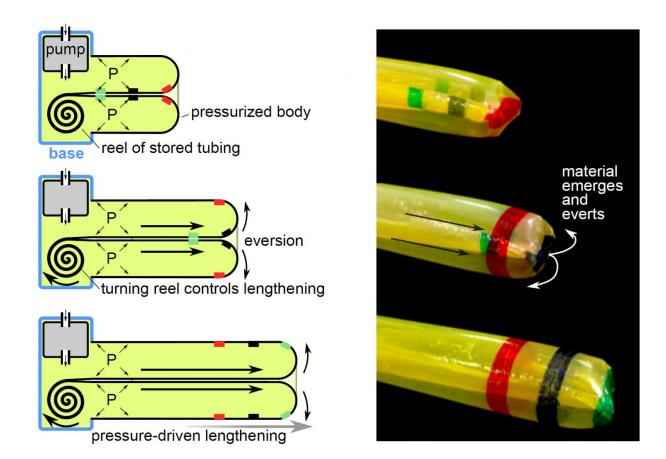
Unfurling from the inside, this robot grows from a 0.28-meter reel of flattened polyethelene plastic tubing to a 72-meter tube. The robot can reverse its growth as well, by decreasing air pressure inside it. Credit: Hawkes et al., *Sci. Robot.* 2, eaan3028 (2017)
