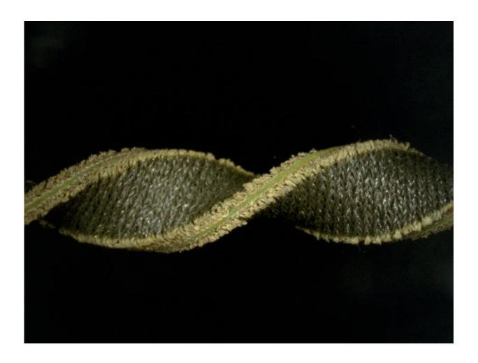
The silicone-textile hybrid sensors are highly flexible and resilient, making them excellent candidates for sensing body movement. Credit: Wyss Institute at Harvard University
