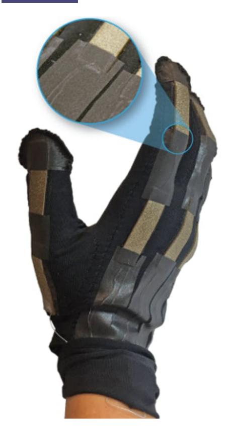
This prototype glove includes soft sensors that are capable of registering movement of each finger individually. Credit: Wyss Institute at Harvard
