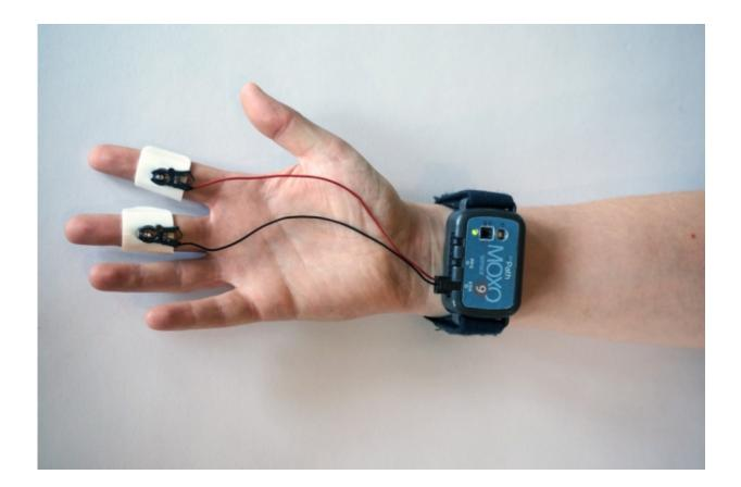
mPath's MOXO sensor, used primarily for market research, is a wearable that resembles a bulky smartwatch. Placed on the wrist, it wirelessly measures changes in skin conductance (subtle electrical changes across the skin), which reflect sympathetic nervous system activity and physiological arousal. Spikes in conductance can signal stress and frustration, while dips may indicate disinterest or boredom. Credit: mPath
