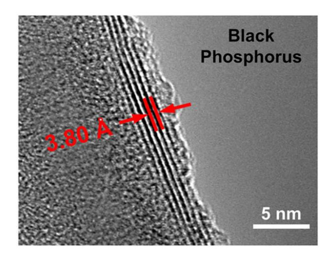
Transmission electron microscope image showing the ultrathin layers of black phosphorus used in the energy harvesting device An angstrom (Å) is about the width of a single atom and is one tenth of a nanometer (nm). Credit: Nanomaterials and Energy Devices Laboratory / Vanderbilt
