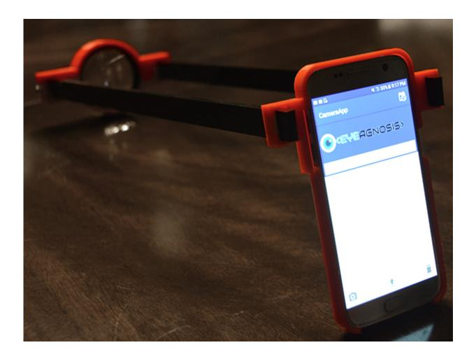
The Eyeagnosis system uses a 3D-printed lens and an AI-enabled smartphone app to diagnose diabetic retinopathy. Credit: Kavya Kopparapu, via IEEE
