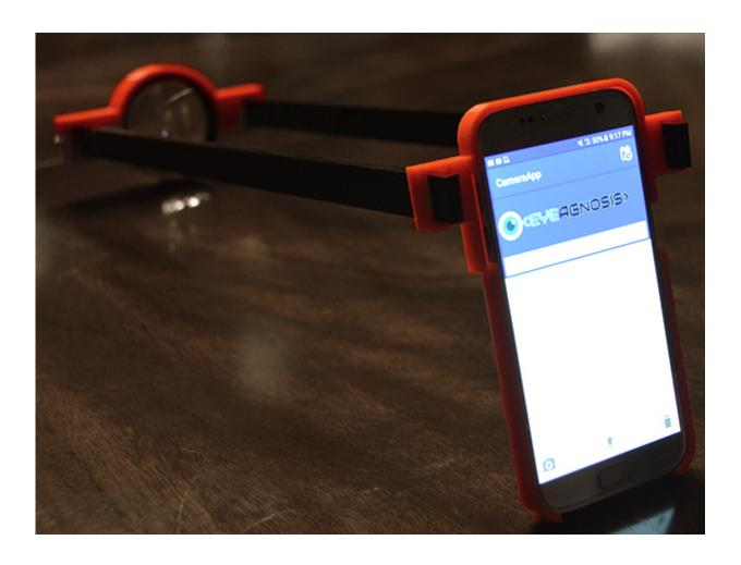
The Eyeagnosis system uses a 3D-printed lens and an AI-enabled smartphone app to diagnose diabetic retinopathy. Credit: Kavya Kopparapu, via IEEE
