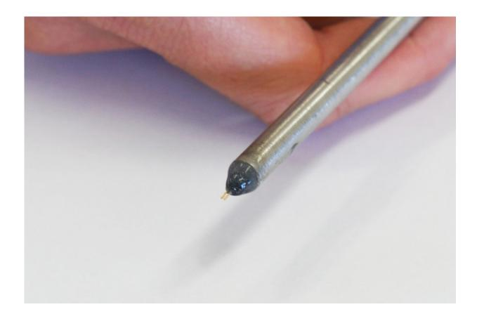
The Conduino's closely-spaced electrodes come from a stripped-down micro USB plug Credit: Sonia Fernandez
