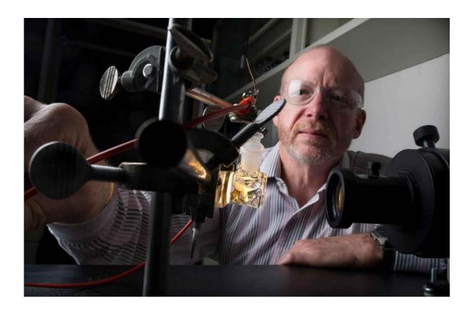
NREL Senior Scientist John Turner tests a photo electrochemical water-splitting system in the hydrogen laboratory at NREL. Turner set a world record for efficiency for the process in 1998 and was part of a team that recently achieved 16.2% solar-to-hydrogen conversion efficiency. Credit: Dennis Schroeder
