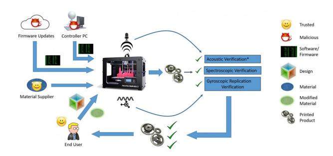
Rutgers University-New Brunswick and Georgia Tech engineers have devised three ways to combat cyberattacks on 3-D printers: monitoring printer motion and sounds and using tiny gold nanoparticles. Credit: Christian Bayens/Georgia Institute of Technology
