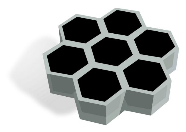
Schematic of a compound solar cell, where a hexagonal scaffold (gray) is used to partition perovskite (black) into microcells to provide mechanical and chemical stability. Credit: Dauskardt Lab/Stanford University
