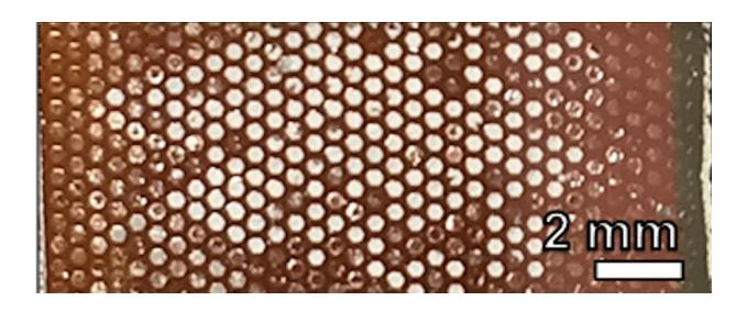
Scaffolds in a compound solar cell filled with perovskite after fracture testing. Credit: Dauskardt Lab/Stanford University
