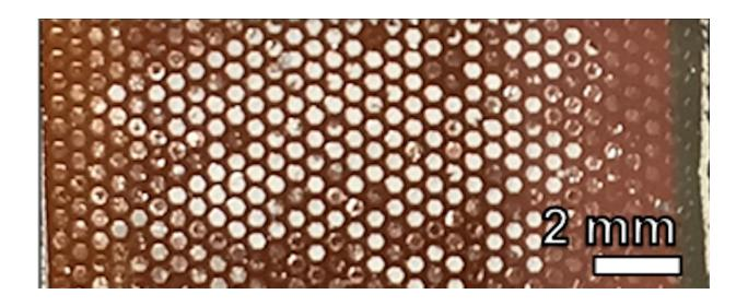
Scaffolds in a compound solar cell filled with perovskite after fracture testing. Credit: Dauskardt Lab/Stanford University
