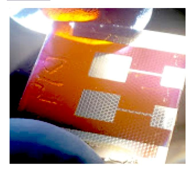
A compound solar cell illuminated from a light source below. Hexagonal scaffolds are visible in the regions coated by a silver electrode. The new solar cell design could help scientists overcome a major roadblock to the development of perovskite photovoltaics. Credit: Dauskardt Lab/Stanford University
