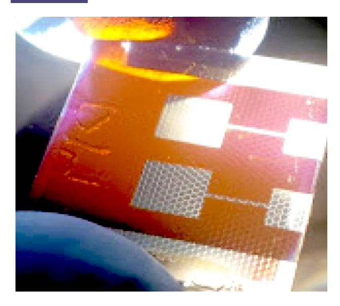
A compound solar cell illuminated from a light source below. Hexagonal scaffolds are visible in the regions coated by a silver electrode. The new solar cell design could help scientists overcome a major roadblock to the development of perovskite photovoltaics. Credit: Dauskardt Lab/Stanford University
