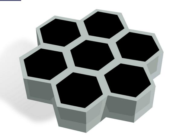
Schematic of a compound solar cell, where a hexagonal scaffold (gray) is used to partition perovskite (black) into microcells to provide mechanical and chemical stability. Credit: Dauskardt Lab/Stanford University
