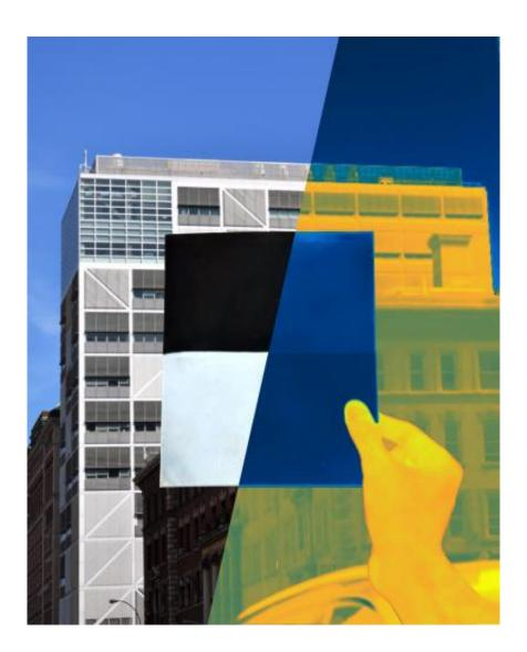
The selective solar absorber (SSA) developed by the researchers appears black and thus absorptive under sunlight (as shown on the photograph on the left). However, for thermal radiation, it behaves like a non-emissive metal mirror (reflecting the dark blue sky, as shown on the thermograph on the right), and
