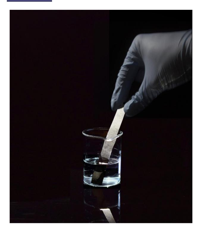
The researchers make their SSAs using a dip-and-dry technique which is considerably simpler than common manufacturing methods for SSAs. Credit: Jyotirmoy Mandal and Yuan Yang / Columbia Engineering
