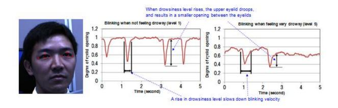
The system extracts an outline of the eyes and monitors time-sequence shifts in blinking features by checking the opening between the eyelids. Credit: Panasonic
