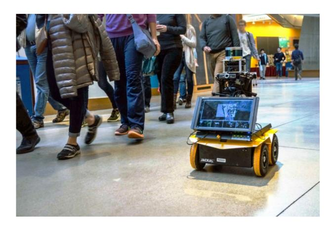
Engineers at MIT have designed an autonomous robot with "socially aware navigation," that can keep pace with foot traffic while observing these general codes of pedestrian conduct. Credit: Massachusetts Institute of Technology
