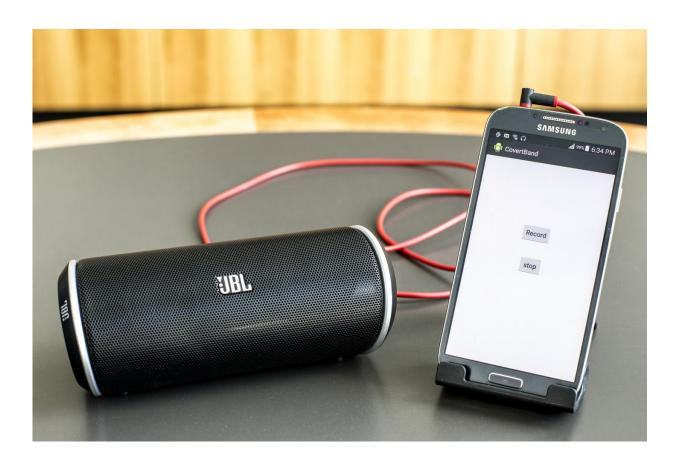
The researchers tested CovertBand using a Samsung Galaxy S4 smartphone hooked up to a portable speaker. Credit: Dennis Wise/University of Washington
