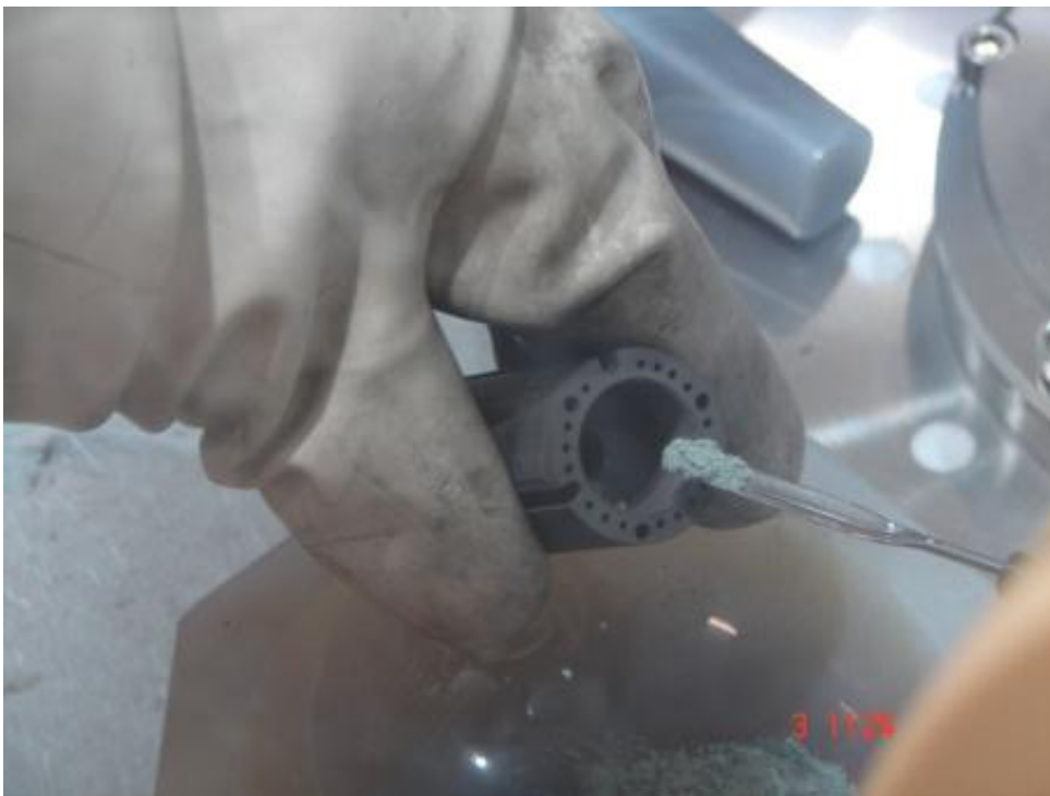
Filling of crucible with sample salt at JRC Karlsruhe
