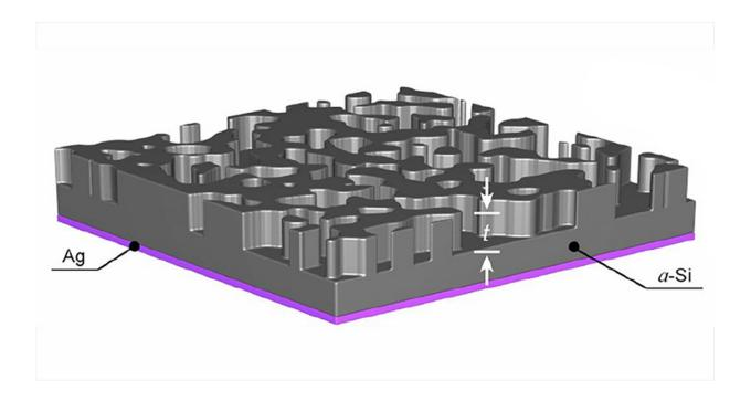
A schematic of quasi-random nanowrinkles on the surface of a silicon wafer. Credit: Northwestern University
