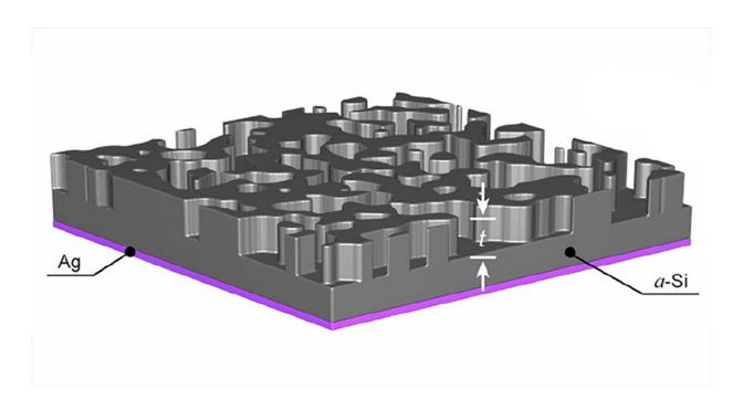
A schematic of quasi-random nanowrinkles on the surface of a silicon wafer. Credit: Northwestern University
