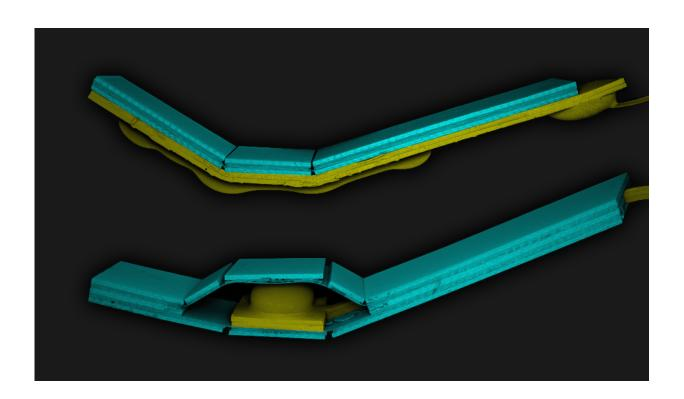
SEM images of the hybrid soft pop-up actuators. The image has been colored in post processing to differentiate between the soft (in yellow) and the rigid structure (in blue) Credit: Wyss Institute at Harvard University
