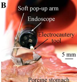
Multi-articulated soft pop-up robotic arm. Concept of the system (left): An endoscope navigating in the GI tract and detail of the arm mounted at the tip of the endoscope. Soft pop-up arm (right) performing tissue counter-traction during an ex-vivo test on a porcine stomach. Credit: Harvard University
