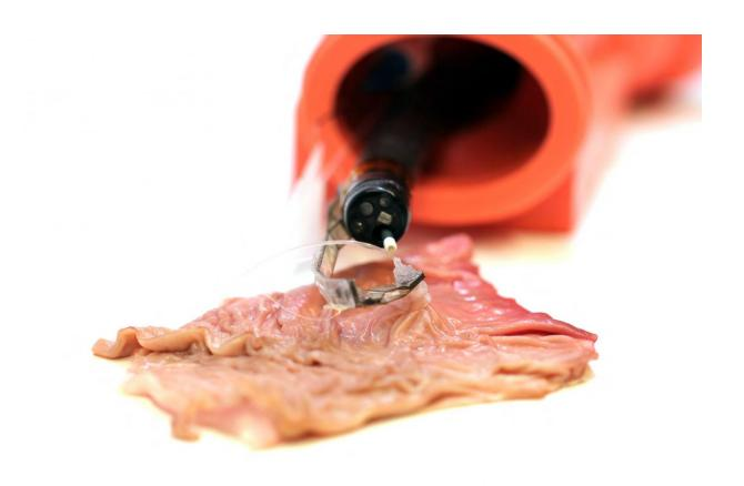
Soft pop-up arm performing tissue counter-traction during an ex-vivo test on a porcine stomach Credit: Harvard University
