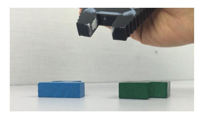
Researchers used their algorithm to design soft grippers with microstructures that can grasp objects by moving their tips when external forces are applied to their extremities. Credit: The Computational Fabrication Group at MIT
