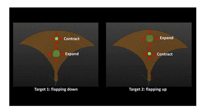
The soft mechanisms for flapping wings are embedded in the material by topology optimization. The wings of the ray are specified to flap up and down when vertices on its spine contract and expand. Credit: The Computational Fabrication Group at MIT
