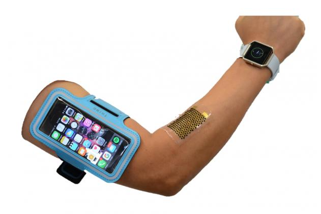
The flexible biofuel cells can power wearable electronics. In the study, researchers used it to power LEDs and a Bluetooth radio. Credit: University of California San Diego
