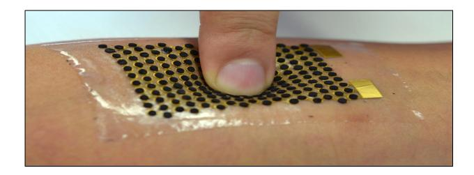
The biofuel cell can stretch and flex, conforming to the human body. Credit: University of California San Diego
