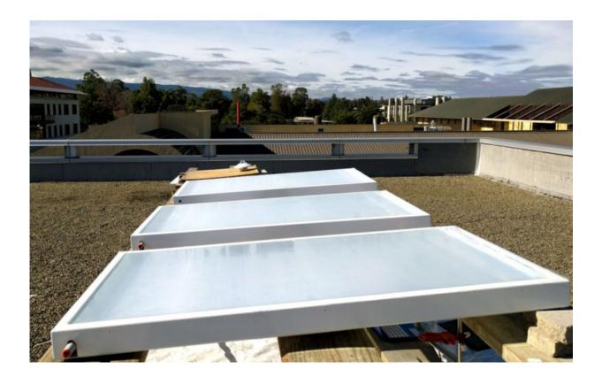
A fluid-cooling panel designed by Shanhui Fan, professor of electrical engineering at Stanford, and former research associates Aaswath Raman and Eli Goldstein being tested on the roof of the Packard Electrical Engineering Building. This is an updated version of the panels used in the research published in *Nature Energy*. Credit: Aaswath Raman
