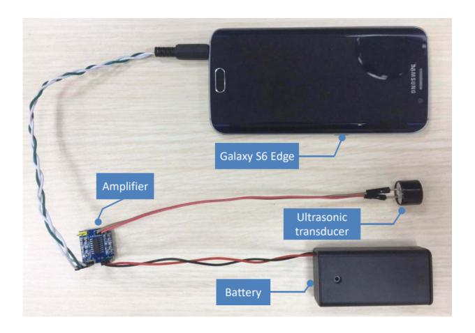
Portable attack implementation with a Samsung Galaxy S6 Edge smartphone, an ultrasonic transducer and a low-cost amplifier. The total price for the amplifier, the ultrasonic transducer plus the battery is less than \$3. Credit: arXiv:1708.09537 [cs.CR]
