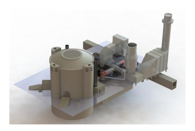
One proposed application of the firebrick-based thermal storage system is depicted in this hypothetical configuration, where it is coupled to a nuclear power plant to provide easily dispatchable power. Credit: Massachusetts Institute of Technology
