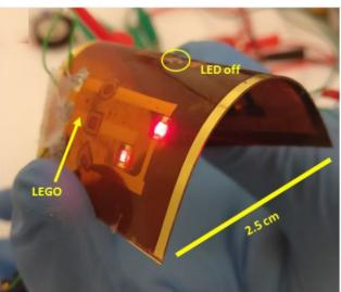
(Left) Lego modules with three different shapes (heart, square, and circle) with the same and different teeth. Scale bar is 5 mm. (Right) Flexibility of an assembled device with Lego-electronics. The LEDs are on where epoxy was applied and off where there is no epoxy. Credit: Shaikh et al. ©2017 Wiley-VCH
