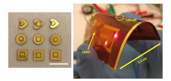
(Left) Lego modules with three different shapes (heart, square, and circle) with the same and different teeth. Scale bar is 5 mm. (Right) Flexibility of an assembled device with Lego-electronics. The LEDs are on where epoxy was applied and off where there is no epoxy. Credit: Shaikh et al. ©2017 Wiley-VCH
