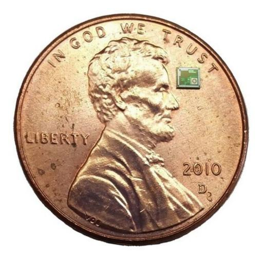
The ATOMS device seen next to a penny. The device has a surface area of 1.4 square millimeters, 250 times smaller than a penny. Credit: Shapiro and Emami Labs/Caltech
