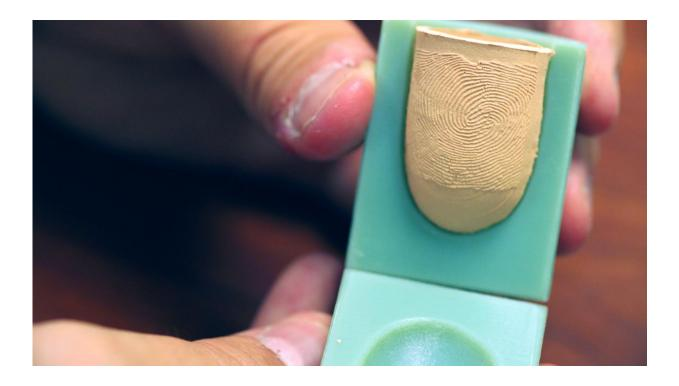
MSU's biometrics expert Anil Jain and his Ph.D. student Joshua Engelsma have, for the first time, designed and created a fake finger containing multiple key properties of the human skin. Commonly called a spoof, this fake finger is being used to test fingerprint readers to help determine their resilience to spoof attacks and which will lead to more resilient fingerprint readers. Credit: Michigan State University
