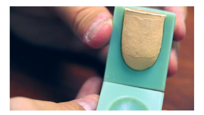
MSU's biometrics expert Anil Jain and his Ph.D. student Joshua Engelsma have, for the first time, designed and created a fake finger containing multiple key properties of the human skin. Commonly called a spoof, this fake finger is being used to test fingerprint readers to help determine their resilience to spoof attacks and which will lead to more resilient fingerprint readers. Credit: Michigan State University
