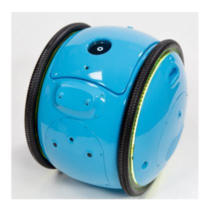
Gita is an autonomous, mobile cargo robot engineered to accompany an individual as he or she navigates through complex indoor and outdoor spaces.
