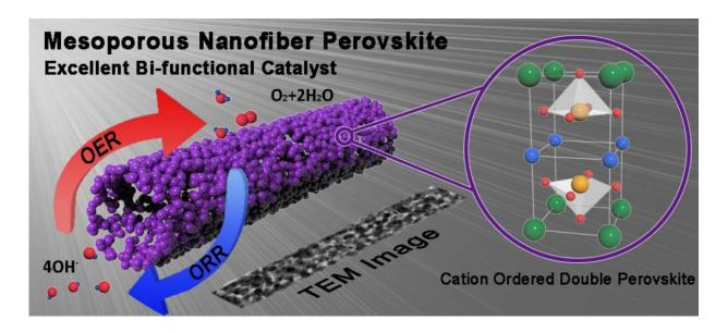
A mesoporous nanofiber of cation ordered perovskite was prepared via electrospinning process, which exhibited notable cell performance and exceptionally high stability for Zn-air battery. Credit: UNIST
