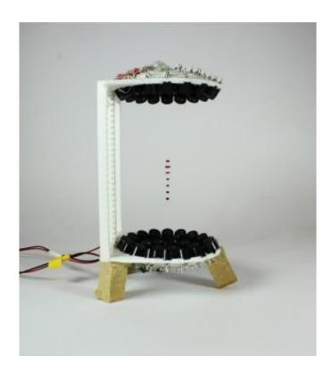
Wine tasting with a difference: droplets of wine are levitated in mid-air and delivered to the user's tongue using sound waves. Credit: University of Sussex
