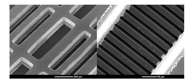
A new electronics-cooling technique relies on microchannels, just a few microns wide, embedded within the chip itself. The device was built at Purdue University's Birck Nanotechnology Center. Credit: Purdue University photo/ Kevin P. Drummond
