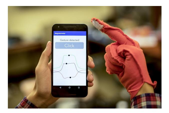
The researchers enabled gesture recognition by sewing the magnetized thread into the fingers of a glove. The phone was able to detect six commonly used interactive gestures with 90 percent accuracy. Credit: Dennis Wise/University of Washington
