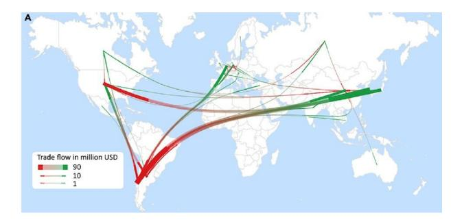
This map shows the aggregated flows of lithium oxide and hydroxide as well as lithium carbonates (does not include concentrates, which would be dominated by Australia). Flows below 1 million USD in value are not included. Credit: Olivetti et al./*Joule* 2017
