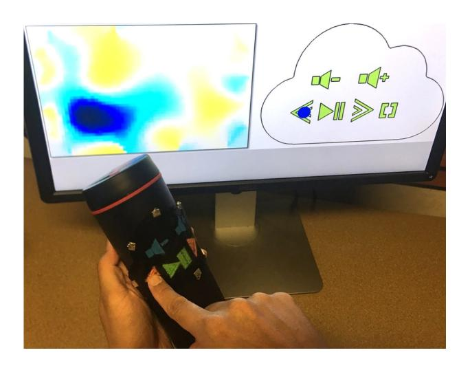
A new type of soft sensor developed at Purdue University can be attached to everyday objects including clothing. Credit: Purdue University image/C Design Lab
