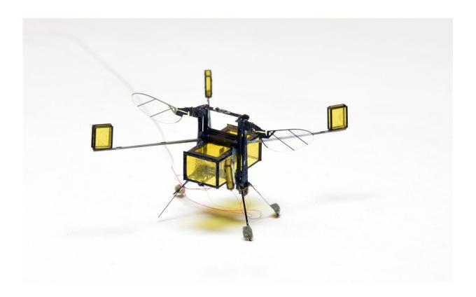
New, hybrid RoboBee can fly, dive into water, swim, propel itself back out of water, and safely land. The RoboBee is retrofitted with four buoyant and a central gas collection chamber. Once the RoboBee swims to the surface, an electrolytic plate in the chamber converts water into oxyhydrogen, a combustible gas fuel. Credit: Yufeng Chen/Harvard SEAS
