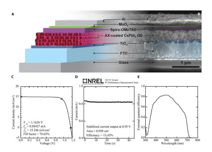
High-efficiency FAI-coated CsPbI3 QDSCs. (A) Schematic cross section of a solar cell. FTO, fluorine-doped tin oxide. (B) SEM image of a device cross section. (C to E) NREL-certified (C) J-V characteristics from forward bias to reverse bias, (D) stabilized current at a constant voltage of 0.95 V, and (E) EQE. Credit: *Science Advances* (2017). DOI: 10.1126/sciadv.aao4204
