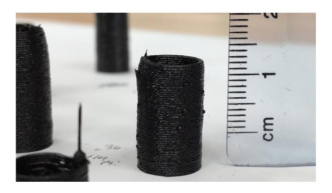
The additive manufacturing process involves depositing thin layers of composite materials on top of each other. AFRL Composite Materials and Processing team researchers used the ultra-bright X-ray at the National Synchrotron Light Source II at Brookhaven National Laboratory to gain better insight into the bonding of composite layers during the additive manufacturing process. Credit: U.S. Air Force photo/Harry Pierson
