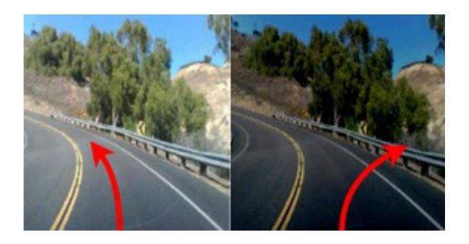
A debugging tool developed by researchers at Columbia and Lehigh generates real-world test images meant to expose logic errors in deep neural networks. The darkened photo at right tricked one set of neurons into telling the car to turn into the guardrail. After catching the mistake, the tool retrains the network to fix the bug. Credit: Columbia Engineering
