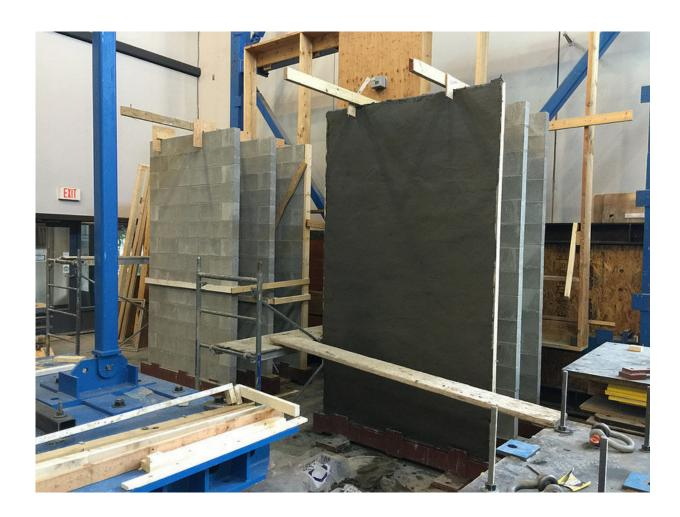
Bare wall, left; EDCC-reinforced wall, right. Credit: UBC
