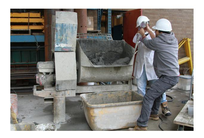
Mixing seismic-resistant concrete at UBC. Credit: UBC
