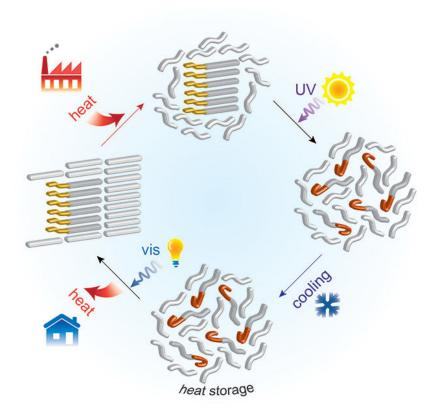
"What we are doing technically," Han explains, "is installing a new energy barrier, so the stored heat cannot be released immediately." In its chemically stored form, the energy can remain for long periods until the optical trigger is activated. Credit: Massachusetts Institute of Technology
