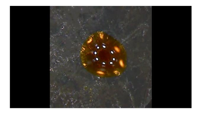
The UV-activated thermal energy storage material shows the rapid crystallization and heat discharge upon visible light (blue LED) illumination. Credit: Grossman Group at MIT
