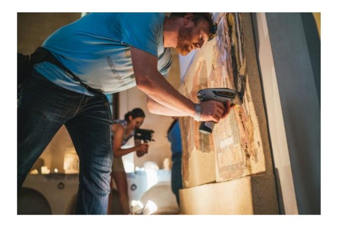
Assistant Professor Admir Masic uses an x-ray fluorescence spectrometer to analyze ancient materials in Italy. Masic is at the forefront of an "antiquainspired" approach to new materials, which considers how ancient successes can be leveraged for the creation of new, sustainable materials. Credit: Lillie Paquette
