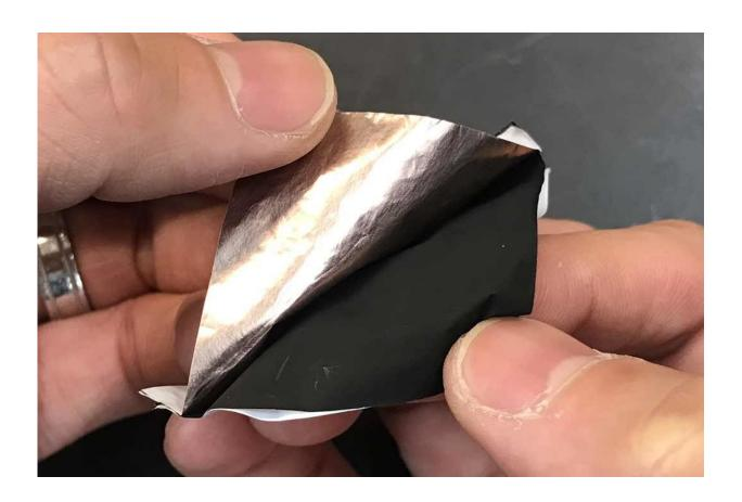
A new textile made from a reversible fabric could warm or cool wearers and keep them comfortable. Two layers of material with different abilities to release heat energy are stacked together and sandwiched between layers of polyethylene. Credit: Yi Cui Group
