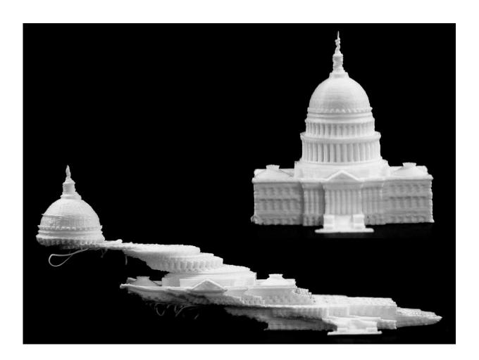
On the bottom, excess vibrations from the 3-D printer caused the printhead to
