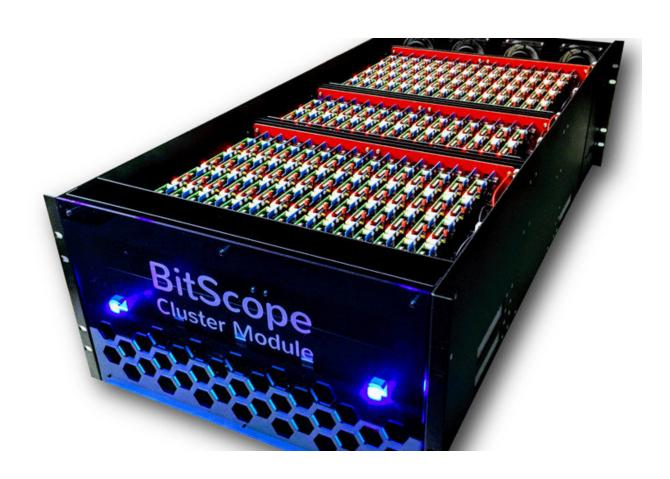
The BitScope Pi Cluster Modules system creates an affordable, scalable, highly parallel testbed for high-performance-computing system-software developers. The system comprises five rack-mounted BitScope Pi Cluster Modules consisting of 3,000 cores using Raspberry Pi ARM processor boards, fully integrated with network switching infrastructure. Credit: Bitscope
