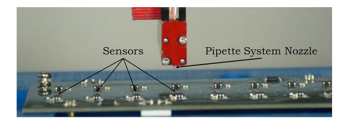
A piezoelectrically actuated pipette system is used as an inexpensive means to detect biological molecules associated with specific diseases, infection or other medical conditions. Purdue University researchers believe the test could be the early detection of traumatic brain injury in athletes, particularly high school football and soccer players. Credit: Purdue University
