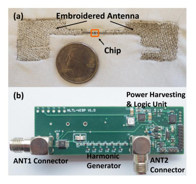
The RFID tag prototypes. (a) An RFID sensor tag chip integrated with the embroidered antenna on fabric. (b) The PCB prototype of the harmonic RFID tag for NCS. Credit: *Nature Methods* (2017). DOI: 10.1038/nmeth.4498
