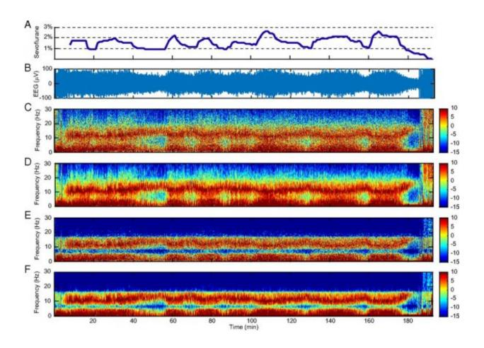
Using a novel analytical method they have developed, MIT researchers analyzed raw brain activity data (B). The spectrogram shows decreased noise and increased frequency resolution, or contrast (E and F) compared to standard spectral analysis methods (C and D). Credit: Seong-Eun Kim et al
