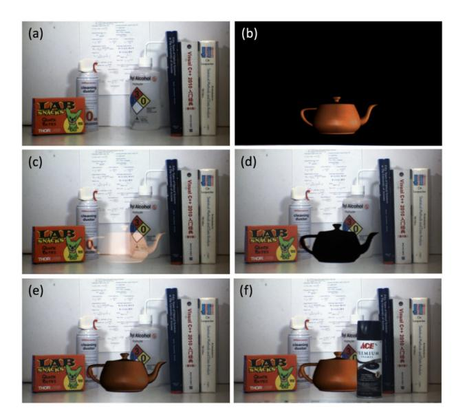
Experimental demonstration of mutual occlusion capability in our OCOST-HMD prototype with photographs captured with a digital camera placed at the exit
