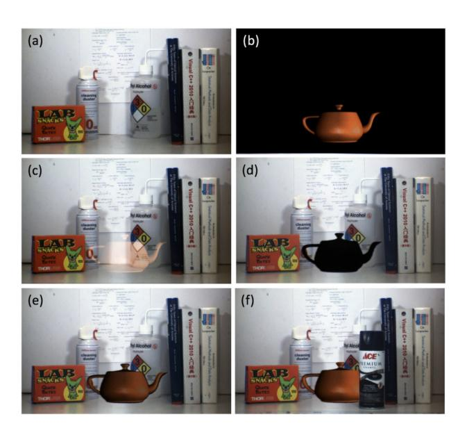
Experimental demonstration of mutual occlusion capability in our OCOST-HMD prototype with photographs captured with a digital camera placed at the exit
