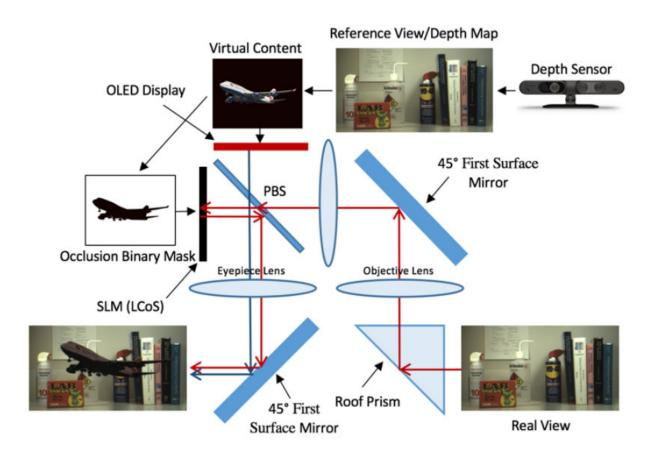
Schematic diagram of the proposed OCOST-HMD design based on two-layer folded architecture. Credit: *Optics Express* (2017). DOI: 10.1364/OE.25.030539
