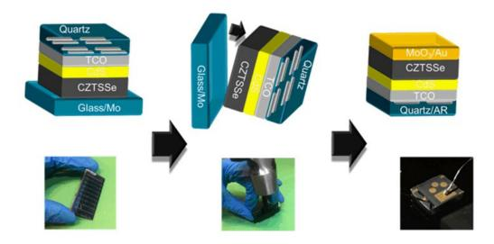
Steps to engineer a new back contact for a kesterite-based solar device. First, an anti-reflective quartz coating is applied to the top of the device (the device will be illuminated through this layer). Next, the substrate and the device are physically separated, i.e. exfoliated, using a hammer. Finally, the new molybdenum/gold back contact is deposited. Credit: Richard Haight, IBM T.J. Watson Research Center.
