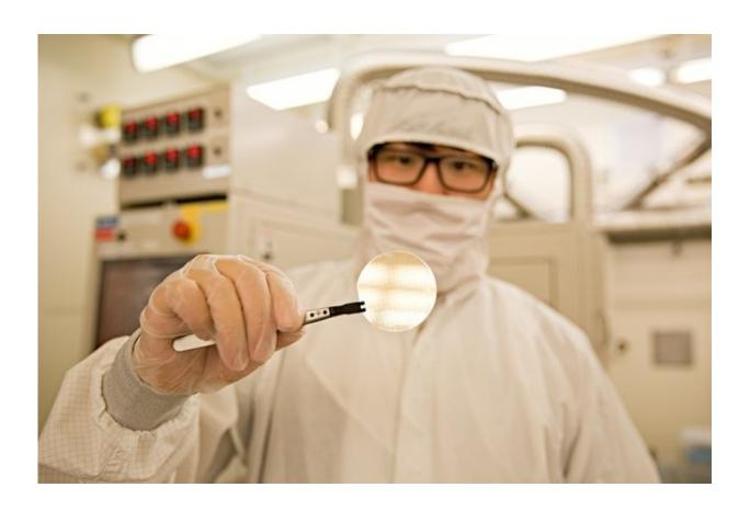
MIT postdoc Yuhao Zhang, handles a wafer with hundreds of vertical gallium nitride power devices fabricated from the Microsystems Technology Laboratories production line. Credit: Yuhao Zhang
