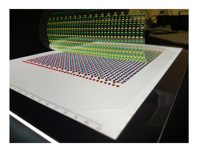
These photos depict the printed, high voltage implementation of the artificial electric organ. We used a 3D bioprinter to deposit arrays of gel precursor droplets onto plastic substrates, and cured them with a UV light to convert them into gels. We printed alternating high-salinity and low-salinity gels (red and blue gels, respectively) onto one substrate, and alternating cation-selective and anion-selective gels (green and yellow gels, respectively) onto a second substrate. When
