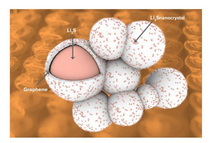
Argonne researchers and their collaborators have brought lithium sulfur batteries closer to reality by creating a new cathode material made of graphene-wrapped lithium sulfide. Credit: Nature Energy
